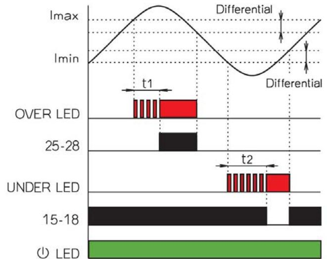
The time delay and differential trip levels help to prevent relay chatter as the monitored current level varies. As the relays have changeover contacts, the relay outputs can be inverted by wiring to the alternative terminals 15-16 or 25-26.
