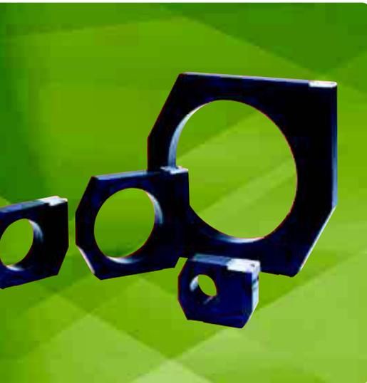
The CBT-94F series of core balanced current transformers are **exclusively for use with our 373-ELR earth leakage protection relay**. The extremely sensitive toroidal core and secondary winding are encapsulated by a self extinguishing case providing excellent mechanical strength, protection from damage and electrical insulation.
