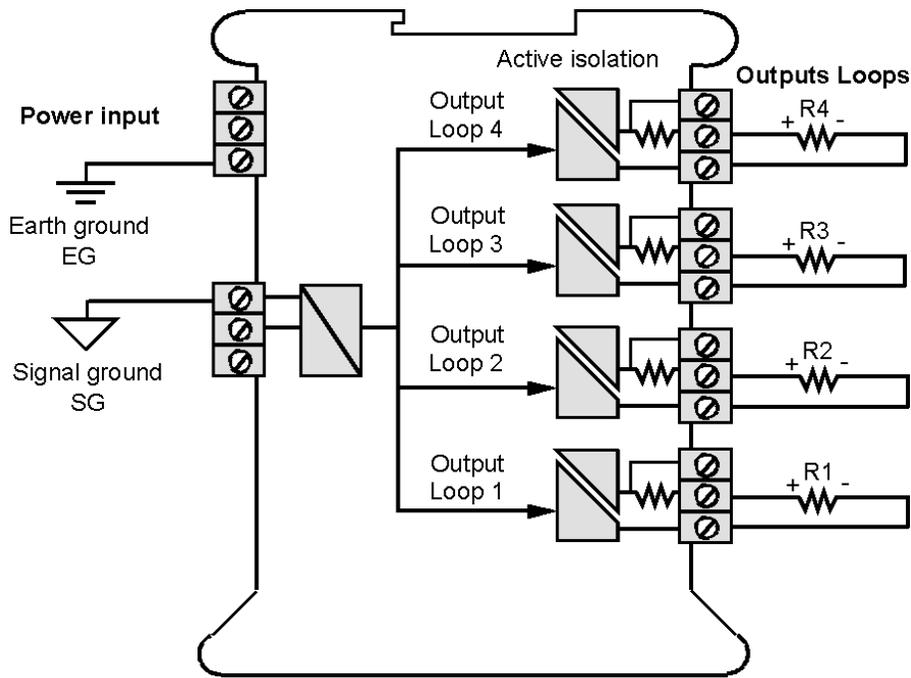
**Floating loads:** Any output load  $R$  that is floating (not connected to a local ground or earth ground) can be connected between current output (Pin 1) and current return (Pin 2). Current return is internally tied to signal ground  $SG$ , which can be floating or be connected to earth ground.
