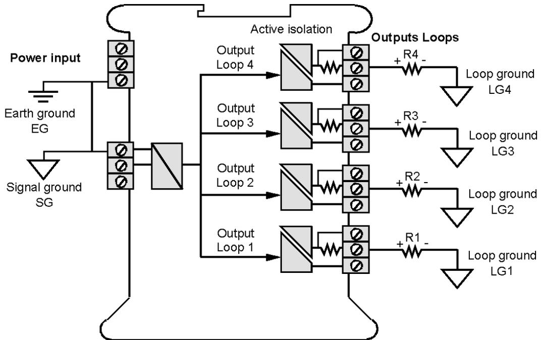
**Grounded loads:** Any output load  $R$  can be connected to a local loop ground  $LG$  instead of current return. The loop grounds  $LG$  can each be different, but can only differ from signal ground  $SG$  by a common mode voltage  $CMV$ , which is defined as  $V_{LG} - V_{SG}$ . Signal ground  $SG$  must be tied to earth ground  $EG$  or be within 1 Volt of  $EG$ .
