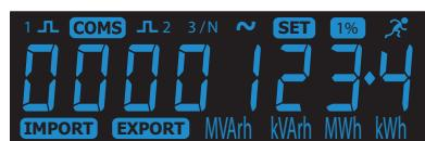
Self-explanatory standard international icons on the display allow to read at a glance what parameters are measured and what system configuration (Wh or VArh) is.
