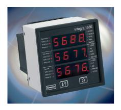
Multi function Integra 1530 digital metering systems provide high accuracy <0.2% measurement, display and communication of all major electrical and power quality parameters, including true RMS system values, power quality data and total harmonic distortion (THD) measurement up to the 31st harmonic.
