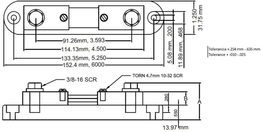
50mv MODEL TYPE FN 1 THROUGH 500 AMPERES
