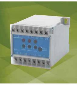
**Speed Sensing** The 250 series speed sensing relay monitors rotating equipment and provides three output contacts which can be used to initiate alarm or shutdown signals. The relay also provides a tachometer output for speed indication. Speed sensing relays are ideally suited for engine and gas turbine monitoring and the protection of generator sets.
