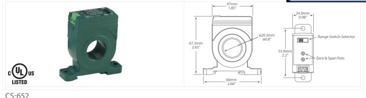
PRODUCT DESCRIPTION The CS-652 Series current sensors monitor line current for electrical loads such as pumps, conveyors, machine tools, or fans and output a 4-20 mA signal to represent the load current. The CS-652 is loop-powered and requires a 15-30 Vdc supply.
