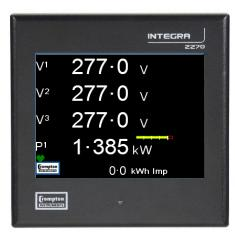
Each of the 5 lines on the display can be defined under the 'User Screen' option in the Setup menu.
