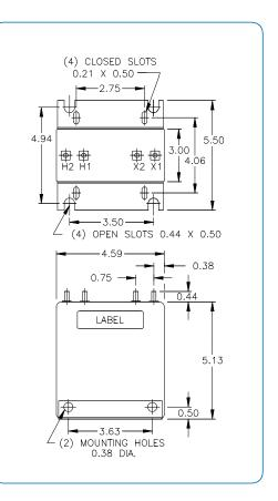
\*\* The circuits of up to five secondaries may be totalized. Equal or unequal line current transformers can be summed with this transformer. Advise the ratios of the line current transformers to be totalized for unequal ratios. Output terminals are X1-X2.
