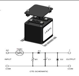
These devices are protected against inadvertent short circuits, input from line surges and inductive kickback from trip coils.
